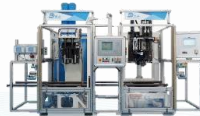
ST190.1/190.2. Press bearing and tighten 2 screws
